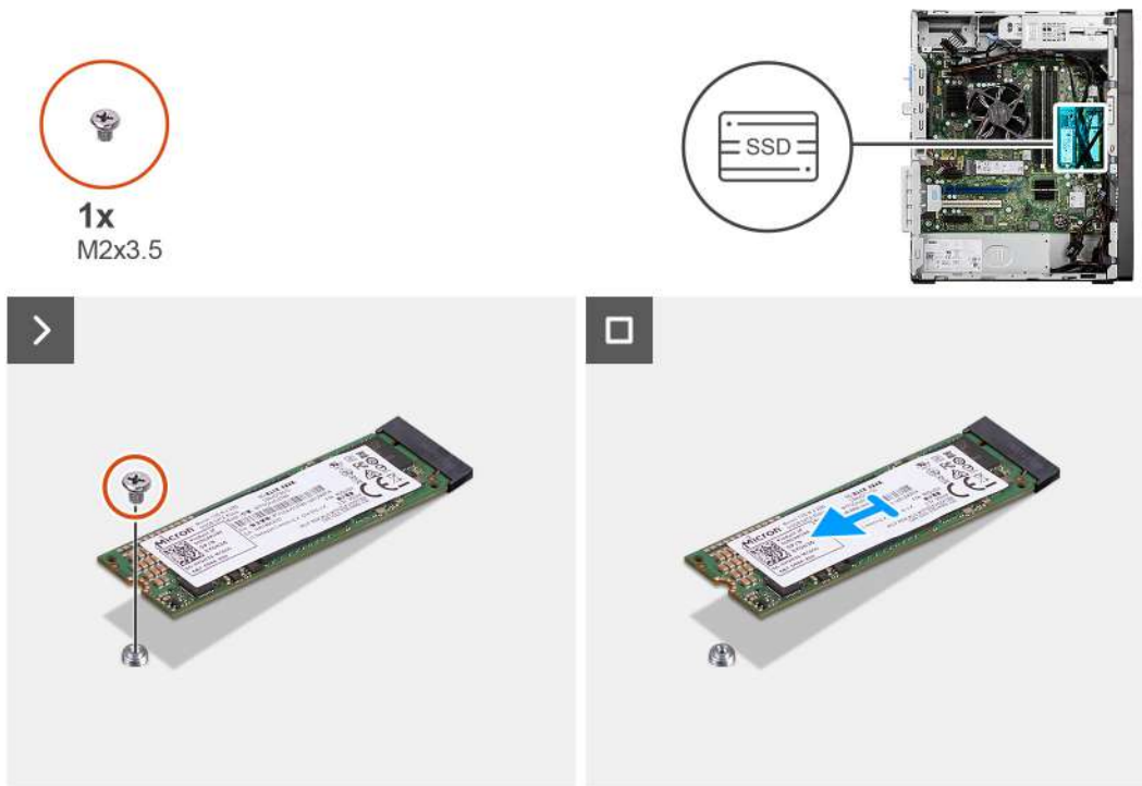
Figure 21. Removing the M.2 2280 solid-state drive
