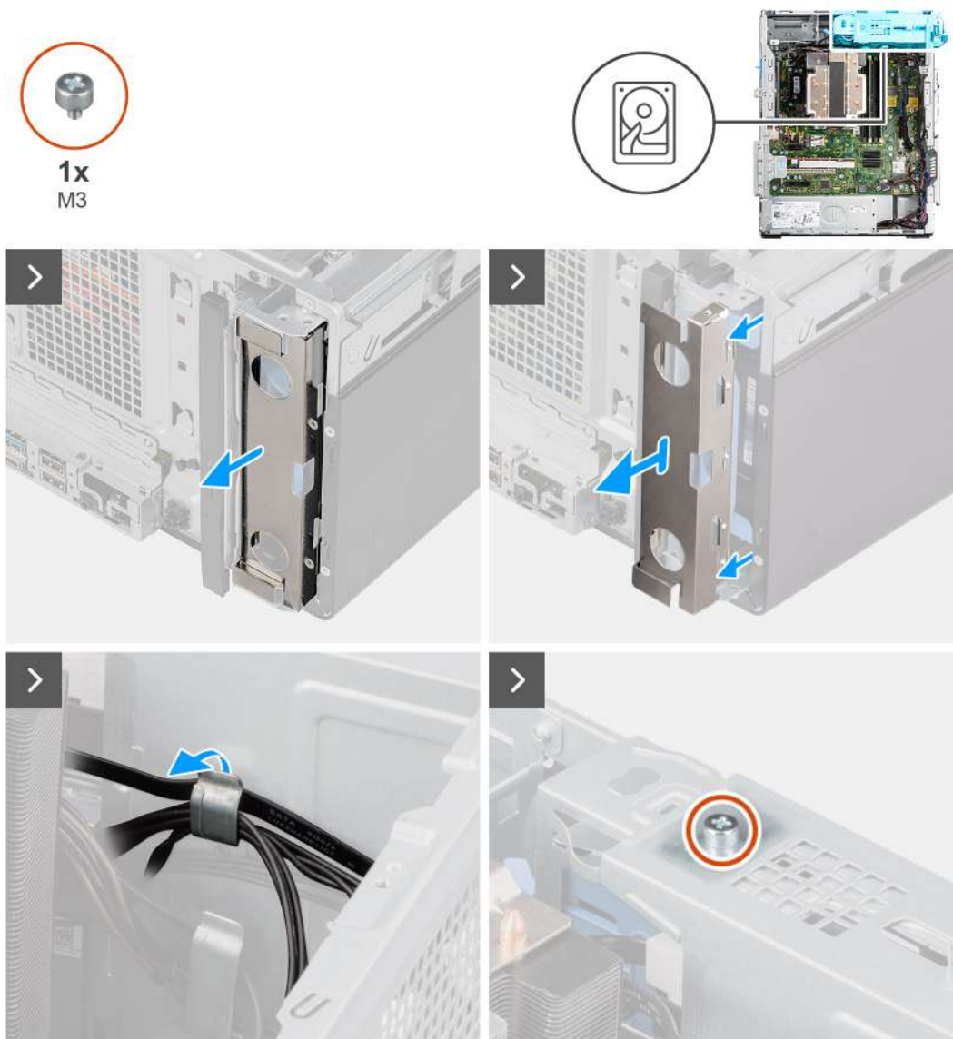
Figure 34. Removing the 3.5-inch hard drive
