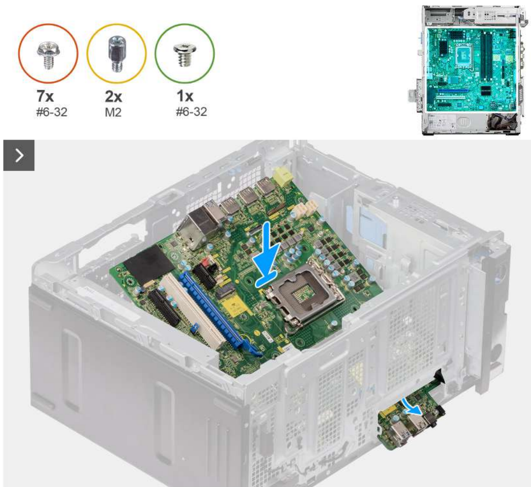
Figure 102. Installing the system board
