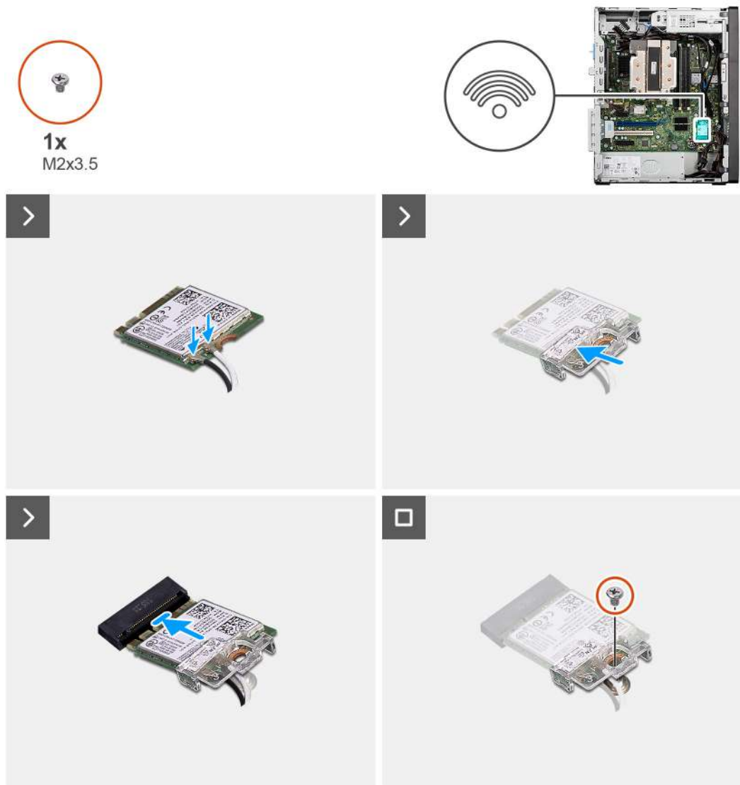
Figure 25. Installing the wireless card
