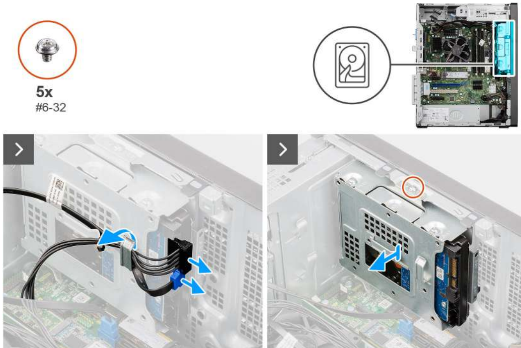
Figure 40. Removing the secondary 3.5-inch hard drive
