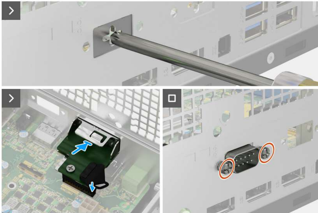
Figure 85. Installing the optional serial module
