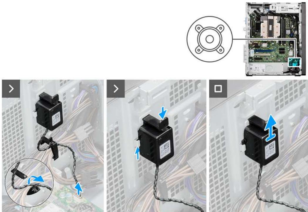
Figure 50. Removing the internal speaker
